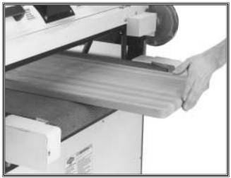
Figure 2. ALWAYS keep fingers away from conveyor and the underside of the stock.
